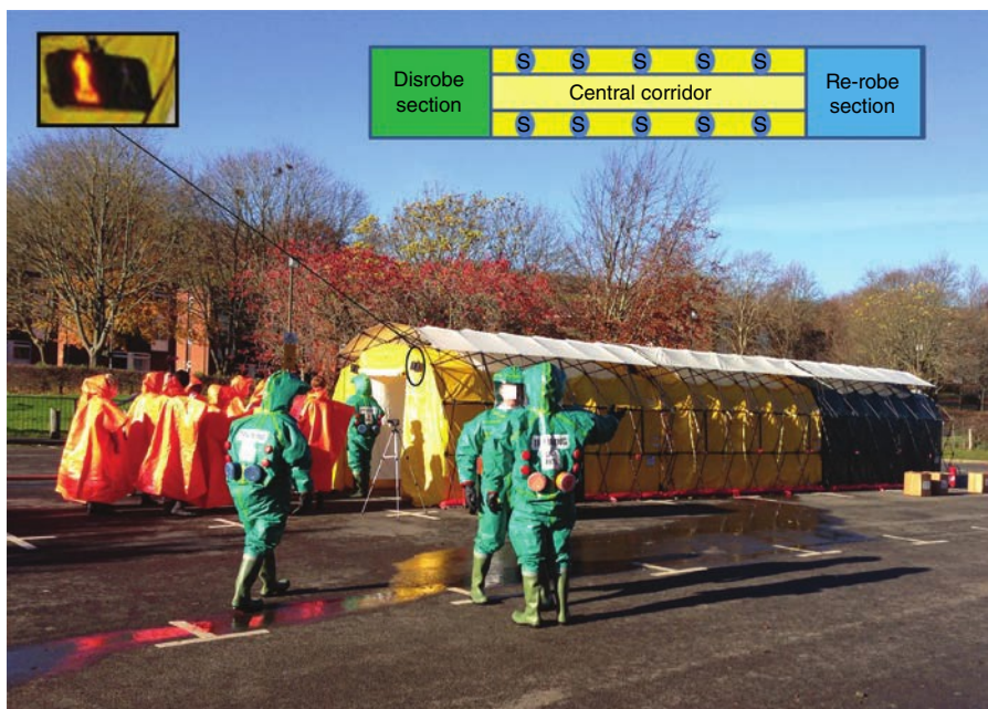
Fig. 15.3. Mass casualty decontamination unit ('MD1') deployed by UK specialist responders. Photograph acquired during an exercise shows a group of ten individuals in high-visibility ponchos (from 'disrobe packs') waiting to enter the unit in accordance with a 'traffic light' system (inset, top left). A schematic of the unit (inset, top right) indicates position of disrobe area, two side corridors (each with five shower areas ('S') for decontamination of ambulant casualties) and a central corridor (used by responders to observe or instruct individuals) which can be adapted for processing non-ambulant casualties. Air heaters and a boiler for shower water are at the rear of the tent and so not shown in this image. (Reproduced with permission of Public Health England © 2013.)
