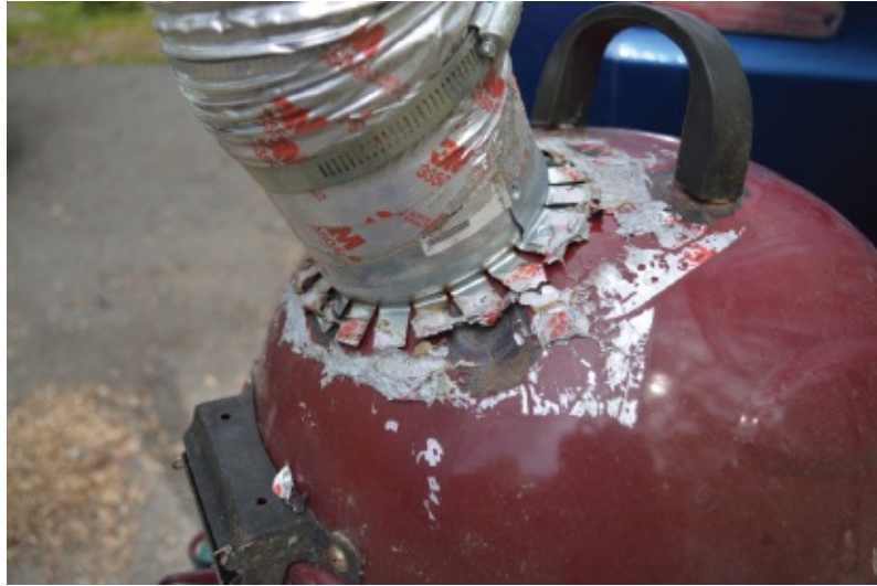
Figure 27.2 Tabs are pulled out and a couple riveted in place.
