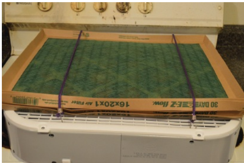
Figure 18.3 Bungee cords tie filters to fan.
