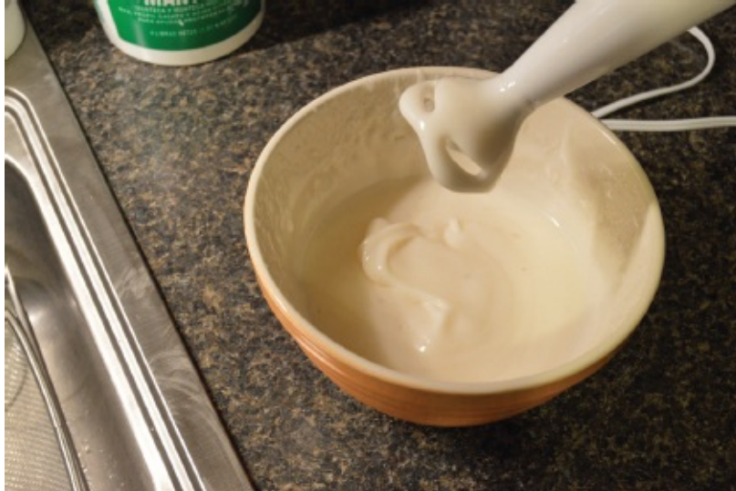
Figure 37.6 Trace is when dribbled soap will leave a trace on the surface of the soap. It is an indicator that the lye and fats are mixed well enough to not separate.
