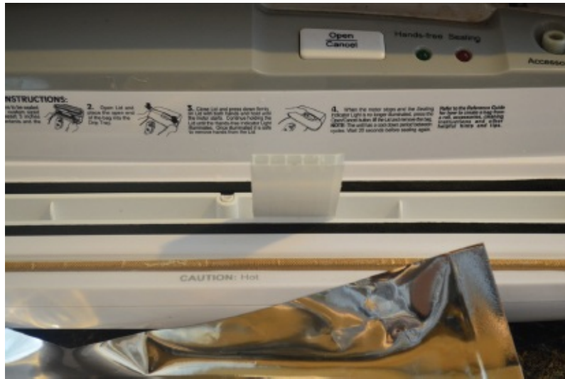
Figure 3.4 Strip must fit into the vacuum chamber of the sealer.
