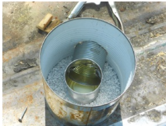
Figure 41.11 Cans A and B inserted in #10 can 18. Push can C into the top of can B, forming a chimney.
