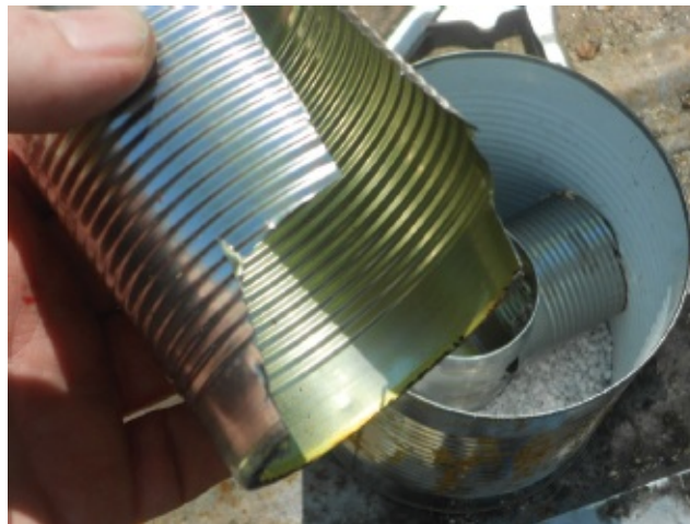
Figure 41.9 Finished cuts on can C
