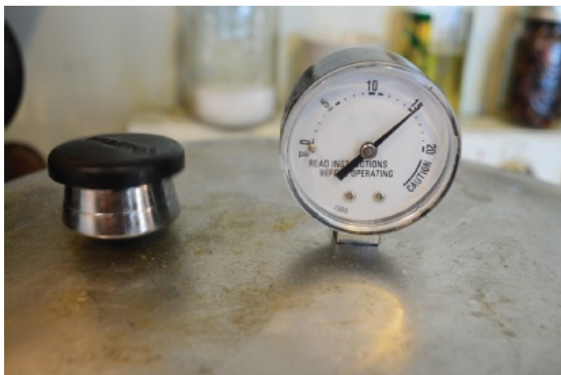
Figure 24.4 Process at 15 psi.
