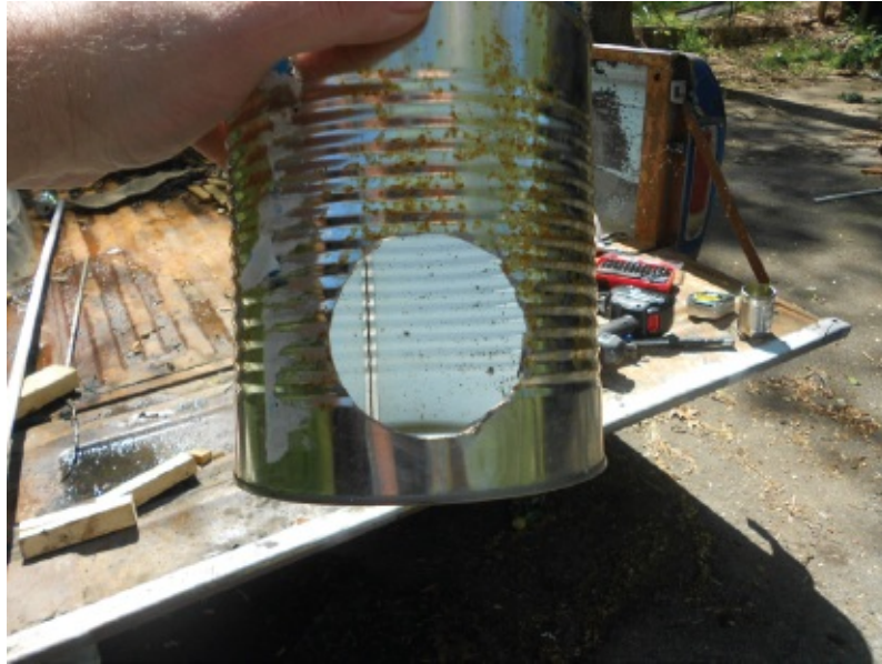
Figure 41.3 Cut a can-sized hole \frac{1}{2} inch from bottom of #10 can.
