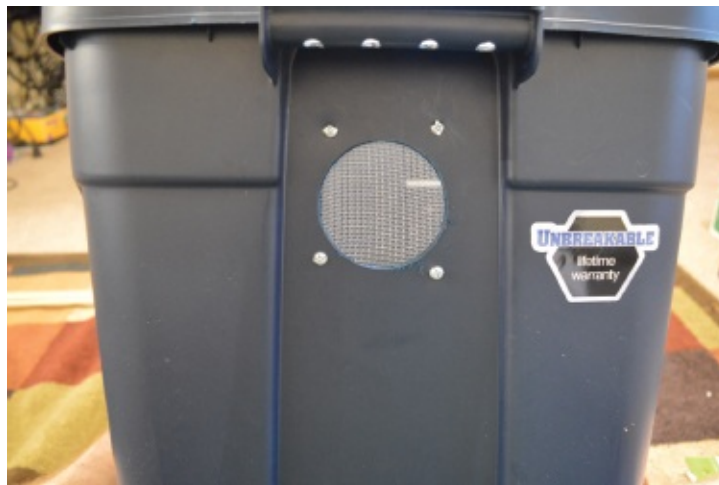
Figure 20.5 Screened vent hole, diagonally situated from inlet fan 6. Affix screen to the fan and the outlet holes to keep flies and other vermin out of the box.
