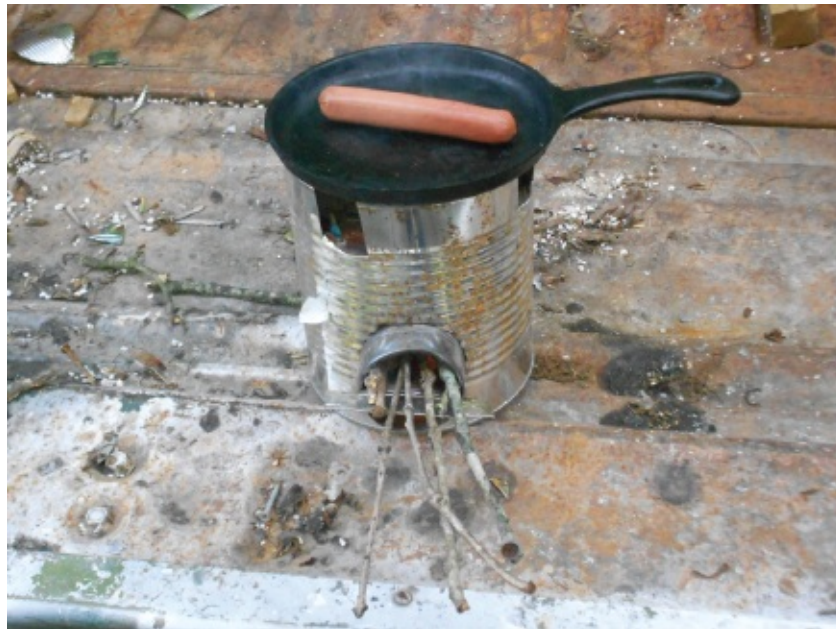
Figure 41.1 Finished rocket stove
