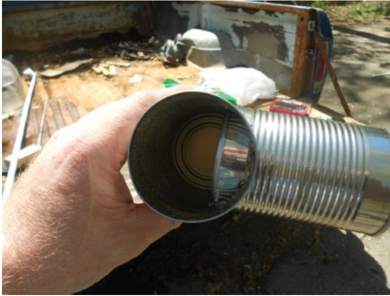
Figure 41.4 Elbow formed by two soup cans
