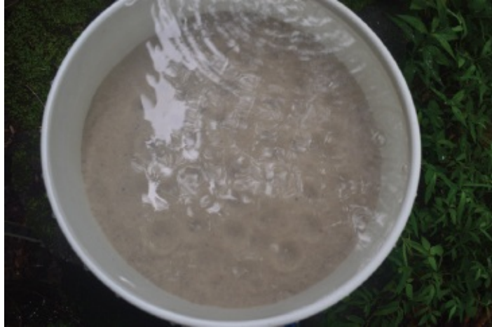
Figure 23.9 The water flow should be gentle enough not to wash away or destroy the bacteria film that will develop over time.
