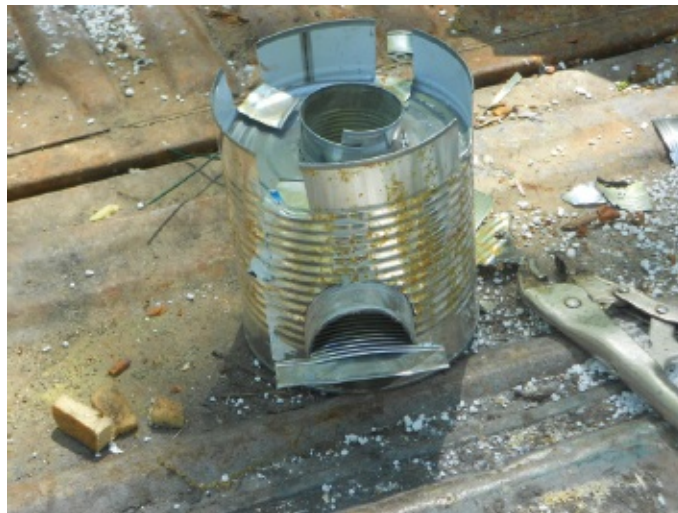
Figure 41.15 Wings keep the “T” in place.
