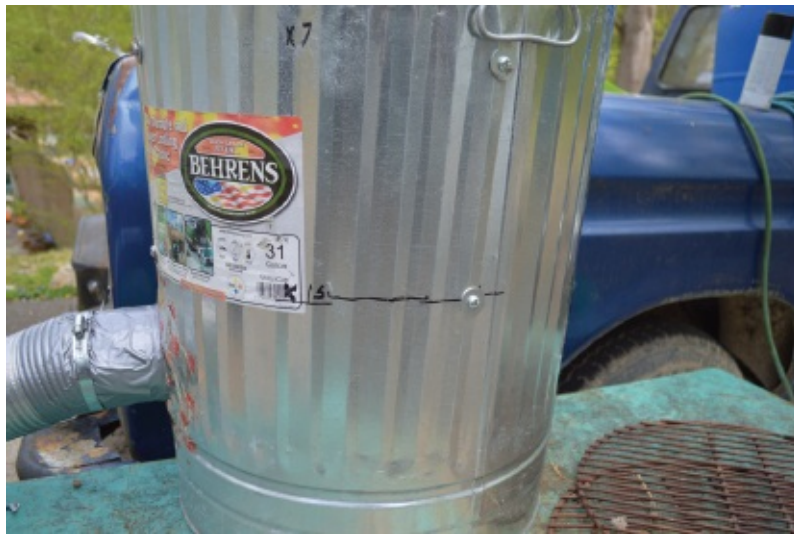
Figure 27.4 To ensure level grates, I marked holes 7 inches from the top lip of the can, and another set 15 inches from the top.
