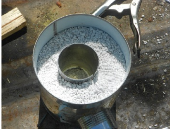
Figure 41.12 Fill with insulation.
